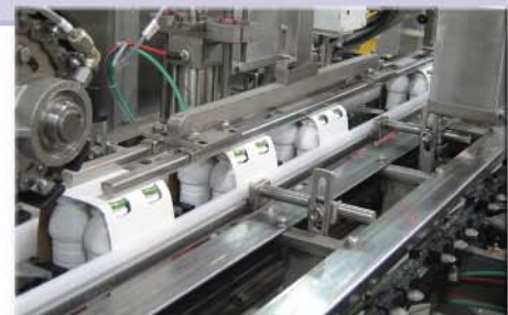
Live sleeve closures and static plows ensure consistently formed sleeves.
