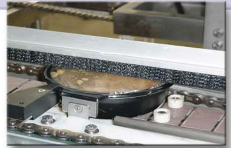
Live belt turning process easily orientates products.
