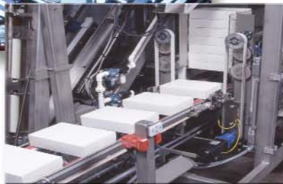
Efficient product metering and accumulation ensure products are gently handled at a variety of speeds.
