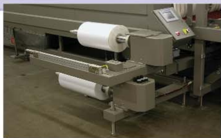
A side film stand simplifies film loading (shown with optional second spindle).
