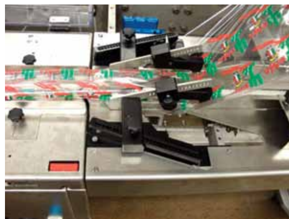
Flexibility The adjustable former option for the Linium 301 means fewer change parts for applications running a variety of products
