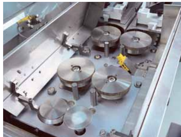
Sanitary Cantilevered infeed and hinged finwheel deck plates allow full access for cleaning and inspection
